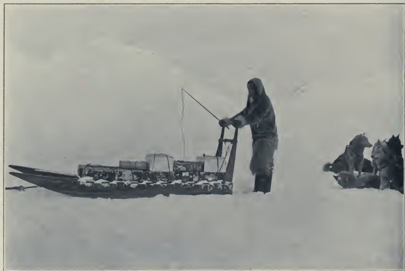
ESKIMO TYPE OF SLEDGE USED ON JOURNEY 9 ft. 6 in. Long, 2 ft. Wide, 8 in High; With Steel Shoes 1½ in. Wide Each has standard load of supplies for team and driver for fifty days— pemmican, biscuit, milk, tea, oil, alcohol
